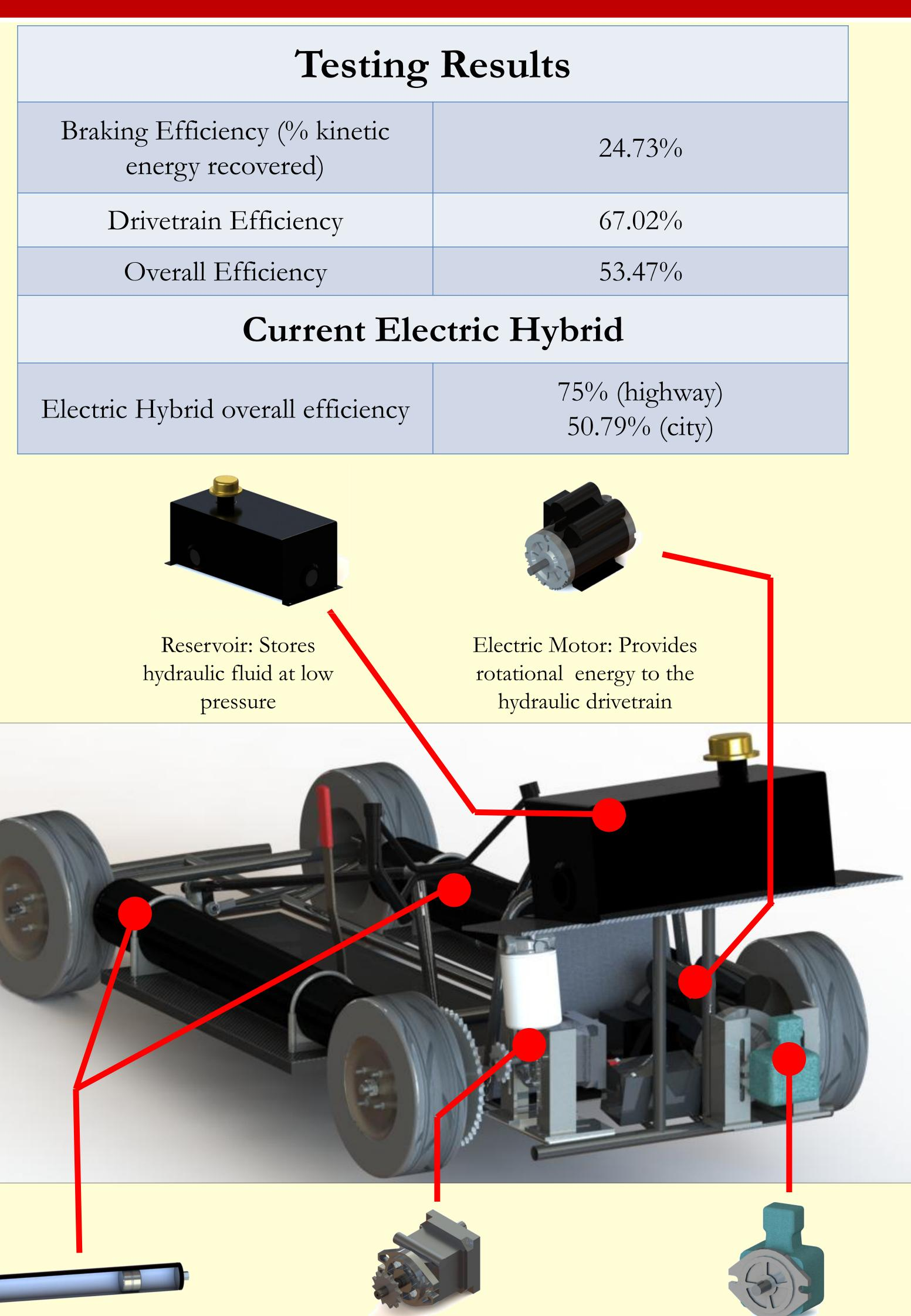
Variable Piston Motor/Pump: Converts high pressure fluid flow to rotational energy to drive wheels; also converts kinetic of the go-kart to high pressure fluid flow during regenerative braking
