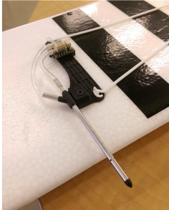
Figure 5: Pitot Airspeed Sensor mounted on wing.
