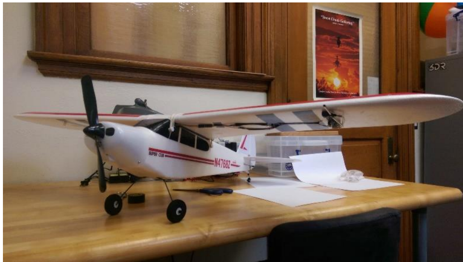
Figure 1: SuperPup with wing-mounted pitot airspeed sensor.
