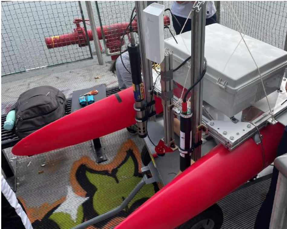
Figure 1: The LISST sensor mounted on the boat.
