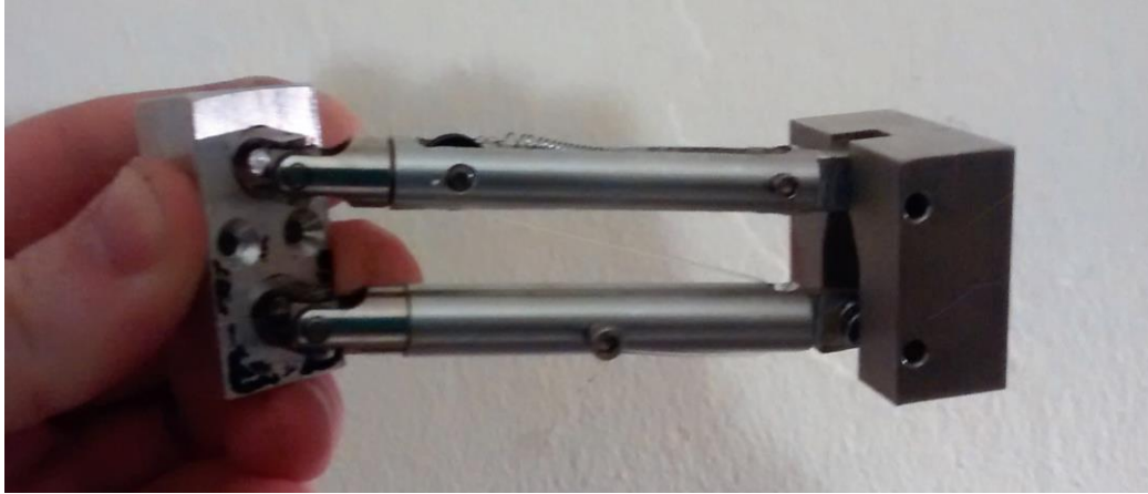
Figure 5: The universal joints at the left are mounted at a 15° downward angle. The slot on the right is wider at the base to allow the planned horizontal motion.
